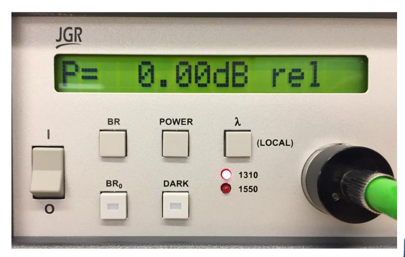
• If the "POWER" button is held long enough then all wavelengths will be referenced. See below. Otherwise do each wavelength being tested individually.
