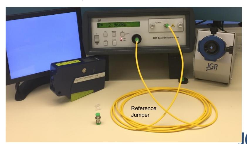
• Press and hold the "POWER" button until a click can be heard. Once the button is let go the meter will read "0.00dB rel" as shown below.
