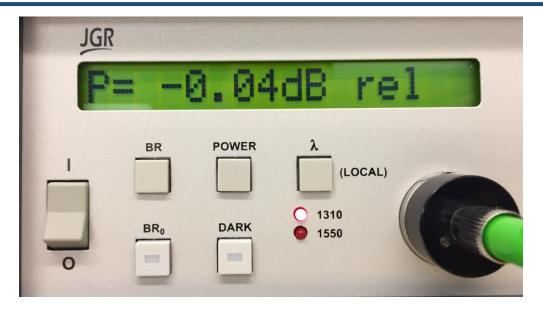
Ensure to inspect each connector (including the end of the reference jumper connecting with the DUT) between each connection. Any dirt or contaminations will cause high IL.
