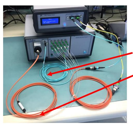
FC/UPC-FC/APC jumper from MS12 output to MS7 common
