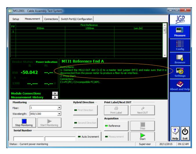
Start part 1 of the reference with the UPC-UPC MTJ disconnected from the detector to produce a fiber-to-air interface (as shown on the previous page).
