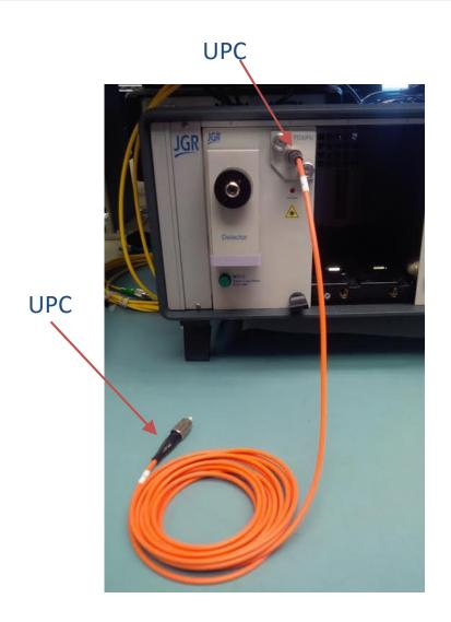
In order to measure the MM APC connector you must perform the first step of the reference with a *CLEAN* 3m UPC-UPC MTJ disconnected from the detector as shown.
