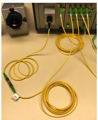
The DUT connector is APC therefore to facilitate the length measurement, a jumper with a PC termination of known length is used.
